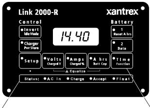
Status lights indicate which cycle the regulator (and/or the charger) is in. The AC light will be OFF if there is no external AC input.
