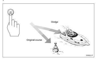
When safely clear of the obstacle, you can reverse the previous course change (for example, press +10 three times), or return to the previous locked heading (LAST HDG).
