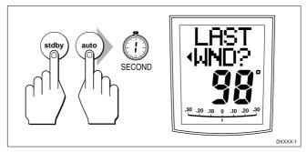
The LAST WND? text alternates with the previous wind angle and direction. The previous locked heading is displayed, with an indicator to show you the direction in which the vessel will turn.
