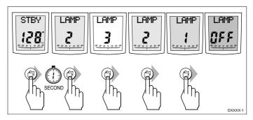
• Subsequent presses of the (1) key cycles the possible illumination settings: L3, L2, L1, OFF, L1, L2, L3 etc. where L3 is the brightest setting.
