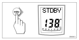
This shows that the control head is active. If the unit does not beep, check the fuse/circuit breaker.
