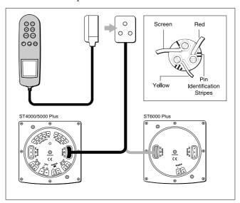
The ST600R can also be connected to any available SeaTalk instrument as well as the autopilot.
