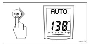
• In Auto mode, the display shows the locked autopilot heading.
