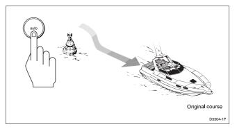
If you do not press **AUTO** while the display is flashing, the current heading will be maintained.
