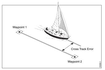
The Large Cross Track Error alarm sounds if the cross track exceeds 0.3nm.
