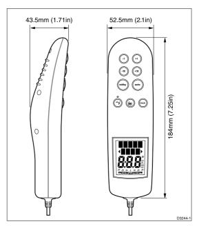
The ST600R remote unit is connected directly to Raymarine autopilots or instruments using the Raymarine data interface system (SeaTalk bus).
