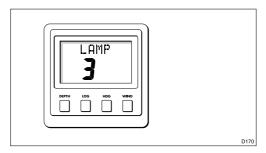
The ST600R should immediately respond by switching on its display illumination.
