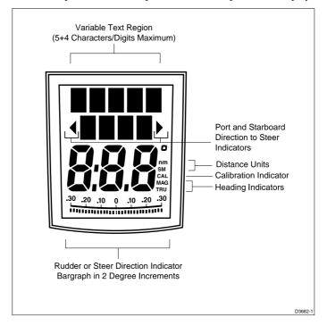
The bar graph at the bottom of the display is normally the rudder bar.
