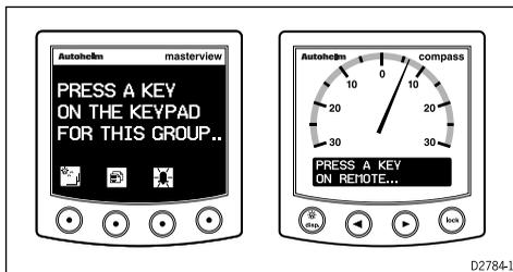
10. Press one of the instrument group keys on the ST7000 Plus to allocate it to the selected group of instruments.
