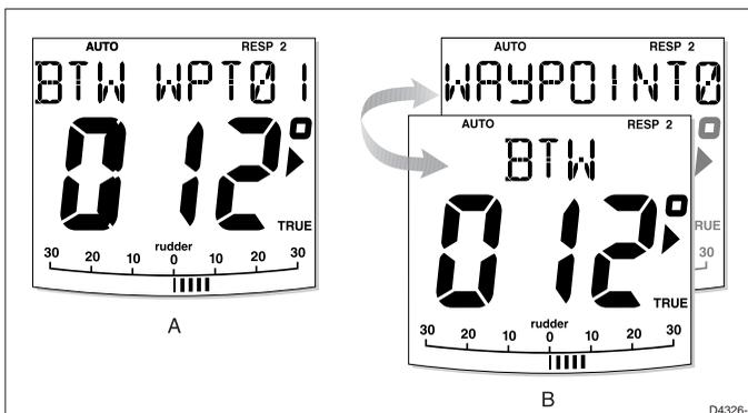
Waypoint names of five characters or less (as at A above) are displayed at the right of the screen. Waypoint names comprising more than five characters (as at B above) are centralised on the screen, alternating with the Data Page name.
