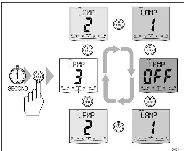
2. Press the **disp** key the necessary number of times to cycle to the required illumination setting. The settings are LAMP 3, LAMP 2, LAMP 1, LAMP OFF, LAMP 1, LAMP 2, LAMP 3 etc, with LAMP 3 being the brightest setting.
