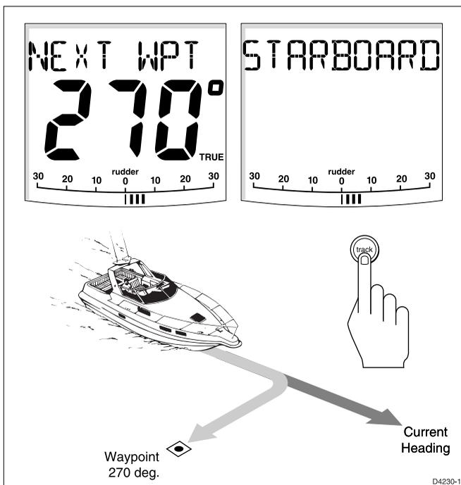
**Note:** If the vessel is further than 0.3 nm from the track, the Large Cross Track Error alarm will sound. Press **standby** to cancel the alarm, hand steer closer to the track, and press **auto** and **track** again.
