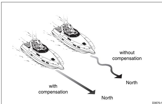
The AutoAdapt feature allows the Course Computer to compensate for heading errors at higher latitudes, which are caused by the increasing dip of the earth's magnetic field. The increased dip has the effect of amplifying rudder response on northerly headings in the northern hemisphere, and on southerly headings in the southern hemisphere.
