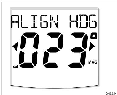
8. Use the **+1**, **-1**, **+10** and **-10** keys, to adjust the displayed heading, until it agrees with the ship's steering compass or a known transit bearing.
