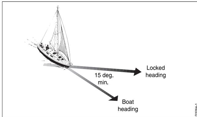
The value must be within the range 15 to 40°, and can be adjusted in 1° steps.
