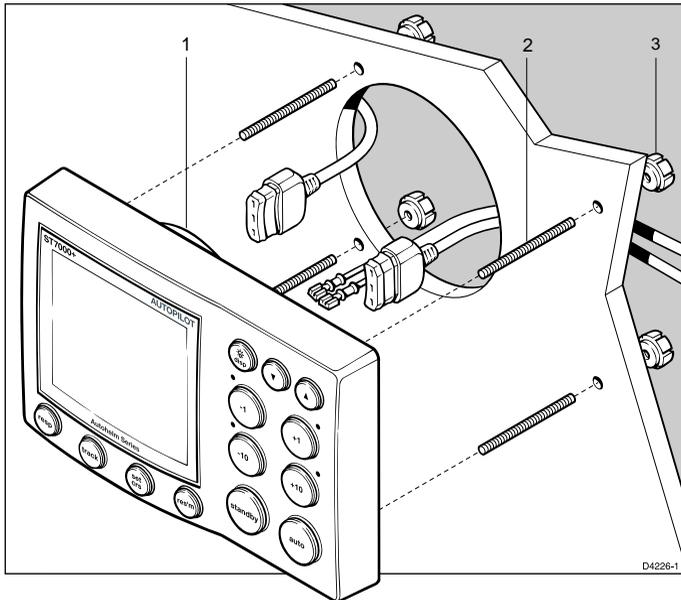
1 Cable boss 2 Fixing studs 3 Thumb nuts
