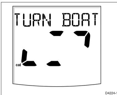
5. Keeping the boat speed below 2 knots, turn the vessel in slow circles. It should take at least 3 minutes to complete 360°.
