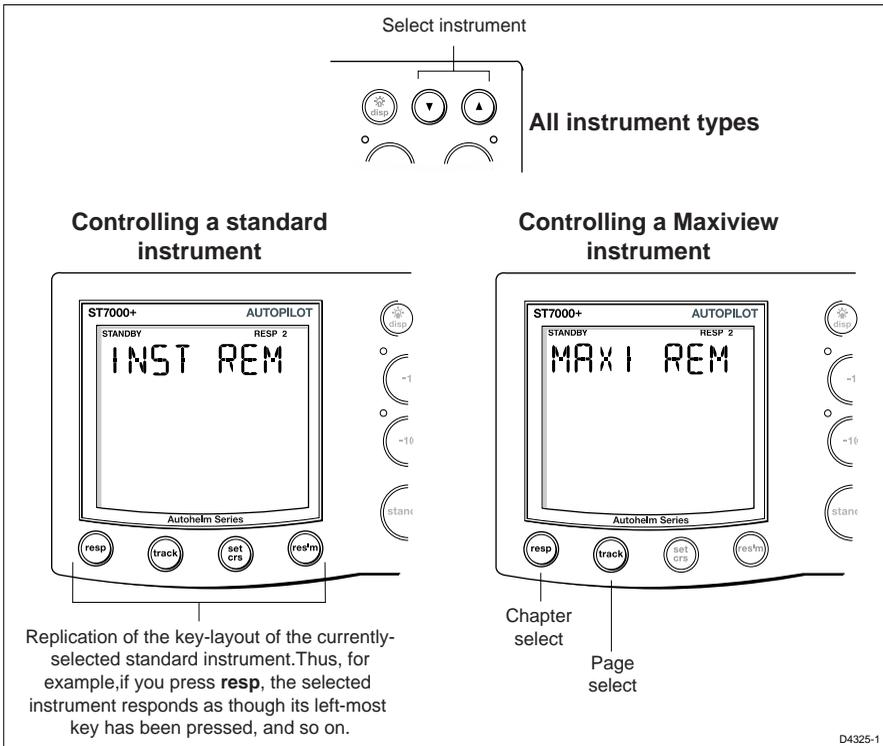
To operate ST60 or ST80 instruments from ST7000 Plus:
